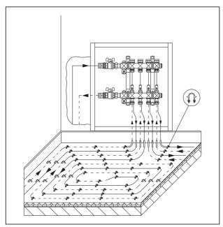
Laying of "Copex", "Copert" and "Copipe" pipes, tacker system
