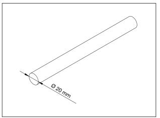
Dimensions round profile made of polyethylene foam
