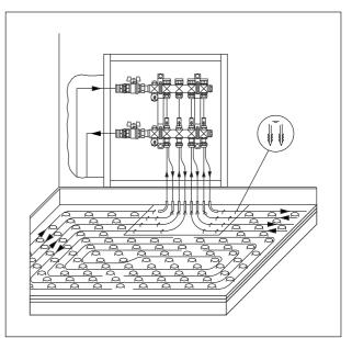
Compensation element in front of the stainless steel distributor/collector "Multidis SF"
