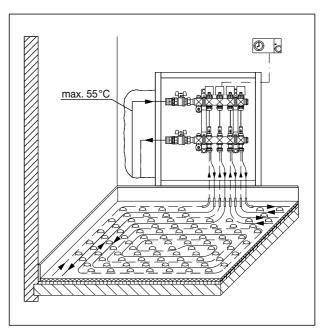
Surface heating system "Cofloor" with stainless steel distributor/collector "Multidis SF"
