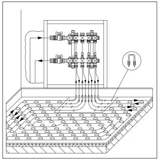
Laying of "Copex", "Copert" and "Copipe" pipes, base mat system
