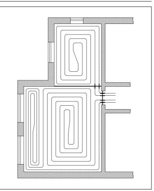
Distribution of heating circuits, positioning of expansion joints
