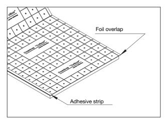
Foil overlap and adhesive strip on base mat and folded board
