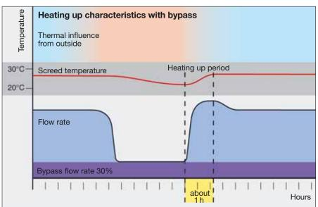
Control capability is the capability of the heating system to react to room temperature modifications.
